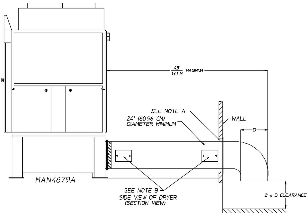
NOTE "A"- OPENING MUST BE 2-INCHES (5.08 CM) LARGER THAN THE DUCT (ALL THE WAY AROUND) THE DUCT MUST BE CENTERED WITHIN THIS OPENING
