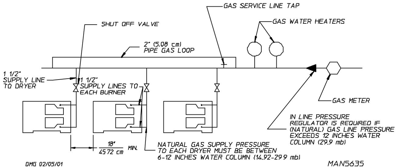
Consistent gas pressure is essential at **ALL** gas connections. It is recommended that a 2-inch (5.08 cm) pipe gas loop be installed in the supply line servicing a bank of dryers. An in-line pressure regulator **must be** installed in the gas supply line (header) if the (natural) gas pressure exceeds 12.0 inches (29.9 mb) of water column (W.C.) pressure.
