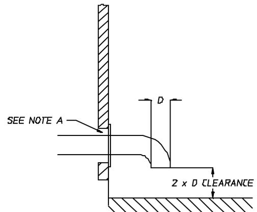
NOTE "A": OPENING MUST BE TWO (2) INCHES (5.08 CM) LARGER THAN DUCT ALL THE WAY AROUND. THE DUCT MUST BE CENTERED WITHIN THIS OPENING
